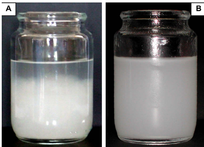
Fig. 4. Aqueous suspension 0.25 % (w/v) of cellulose residue from skin of OFI prickly pear fruit, before (A) and after the Manton Gaulin homogenisation (B).
